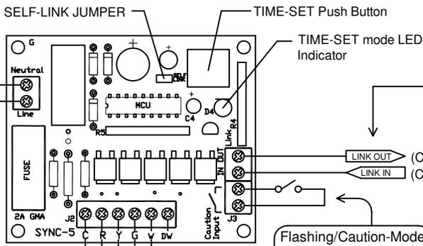
Used when "linking" two or more boards. Remove the "self-link" jumper when linking multiple boards.
