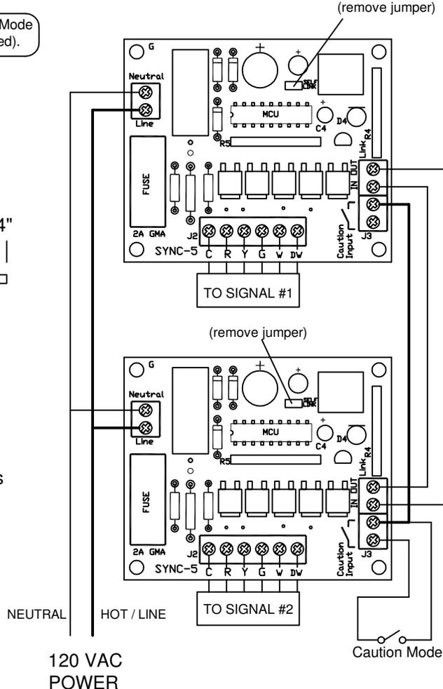
**Warning:** Make sure HOT and NEUTRAL are not reversed on either board. Reversing HOT and NEUTRAL on linked boards will result in damage to both boards.
