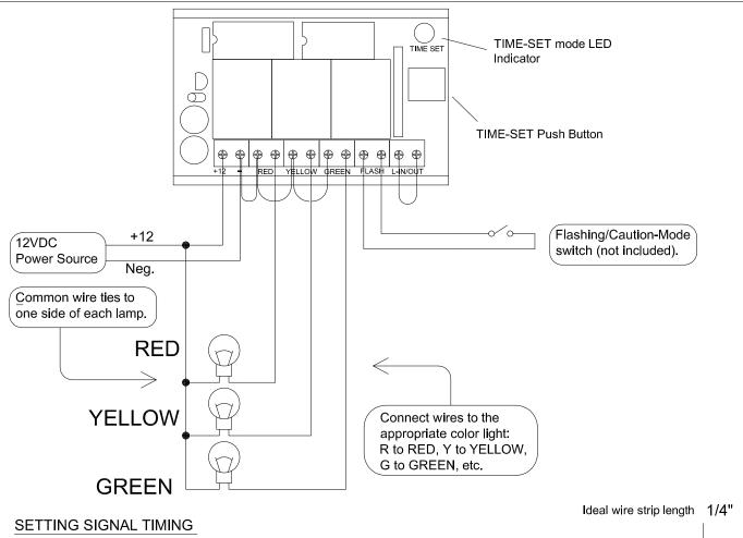
Press and hold the TIME-SET button for approximately 5 seconds until time-set LED lights up then release button. The controller will begin it's normal cycle. Briefly press and release the TIME-SET button when you want to advance to the next step. The board will remember the duration between button presses. Example:
