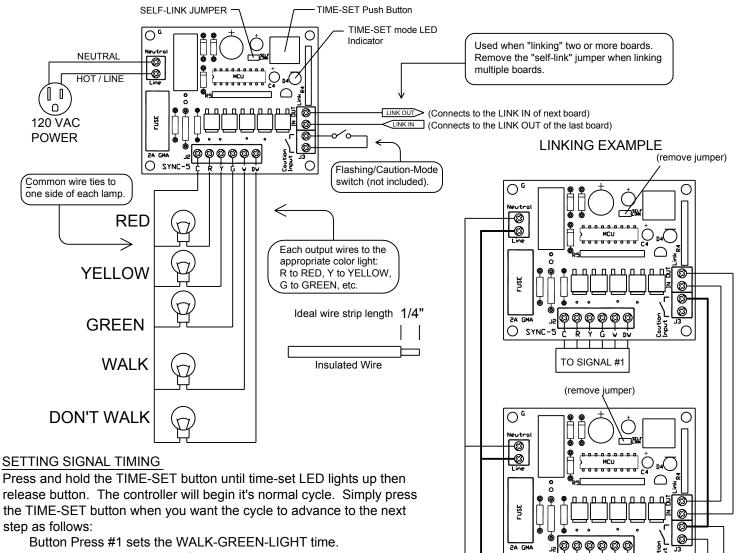
Button Press #2 sets the DON'T-WALK RED Flashing time.
